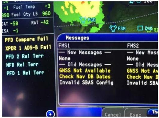
The image shows an avionics display with several error messages. On the left, it lists: 'PFD Compare Fail', 'XPDR 1 ADS-B Fail', 'PFD 2 Rel Terr', 'MFD Rel Terr', and 'PFD 1 Rel Terr'. In the center, there's a weather radar display. On the right, a 'Messages' window is open, showing two columns of messages for FMS1 and FMS2. The messages include: 'New Messages', 'None', 'Old Messages', 'GNSS Not Available', 'Check Nav DB Dates', and 'Invalid SBAS Config'.
