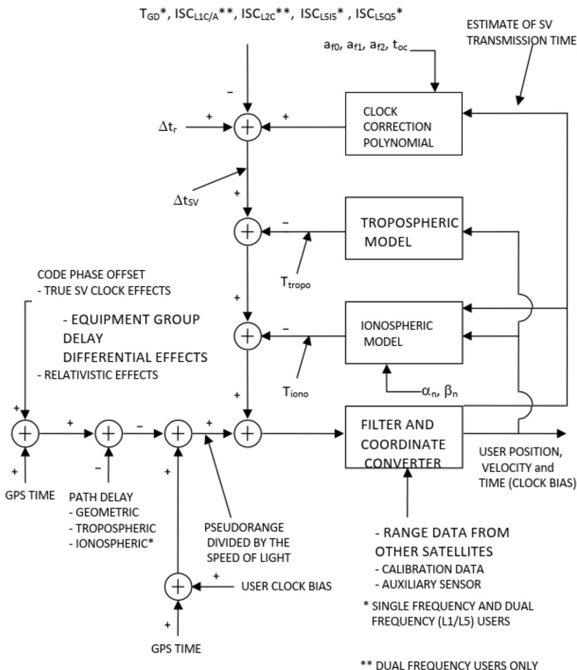
Figure 20-15: Sample Application of Correction Parameters
