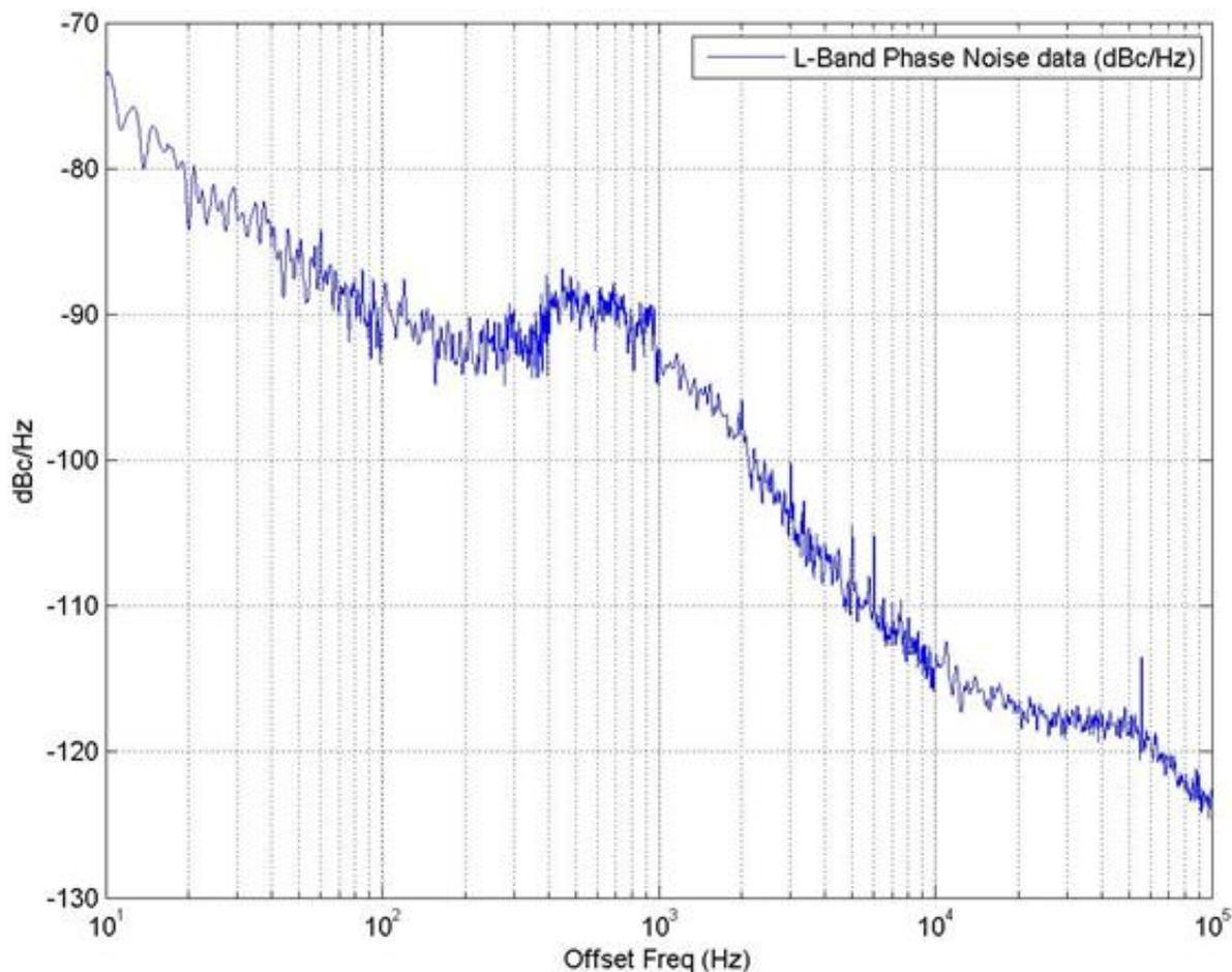
Figure 6-2 Typical GPS III and GPS IIF L5 Carrier Phase Noise Spectral Density
