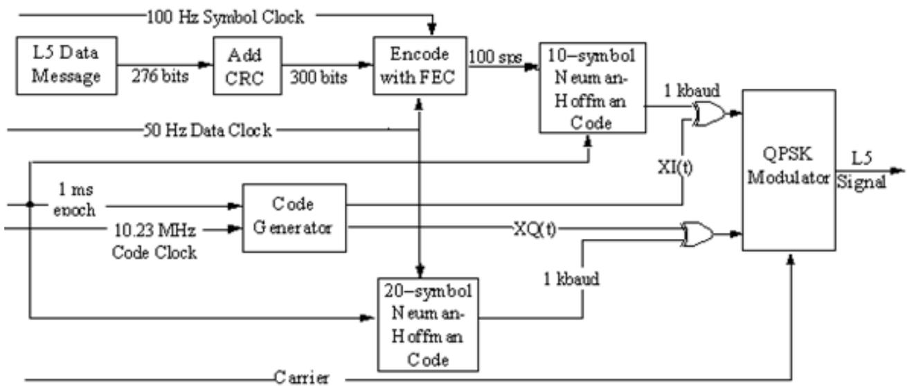
Figure 3-3. Modulation of Signals
