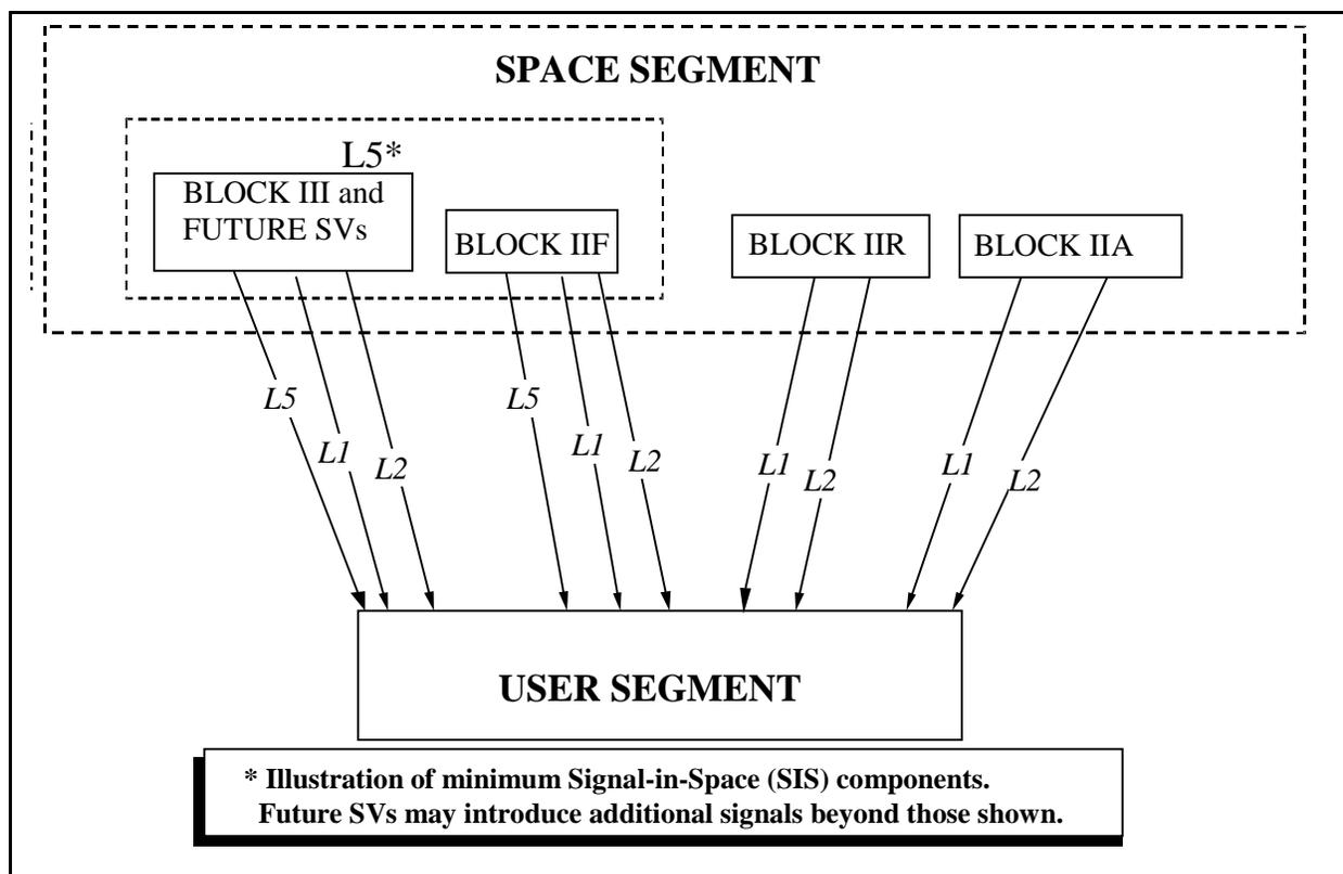
Figure 3-1. GPS Space Segment to User Segment Interfaces
