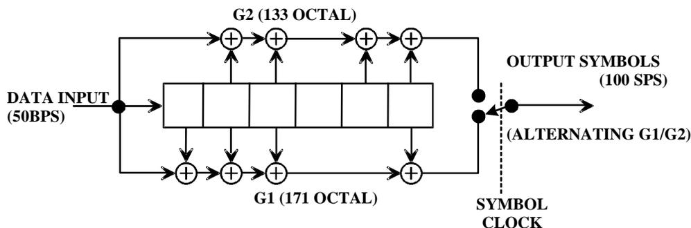
Figure 3-7. Convolution Encoder
