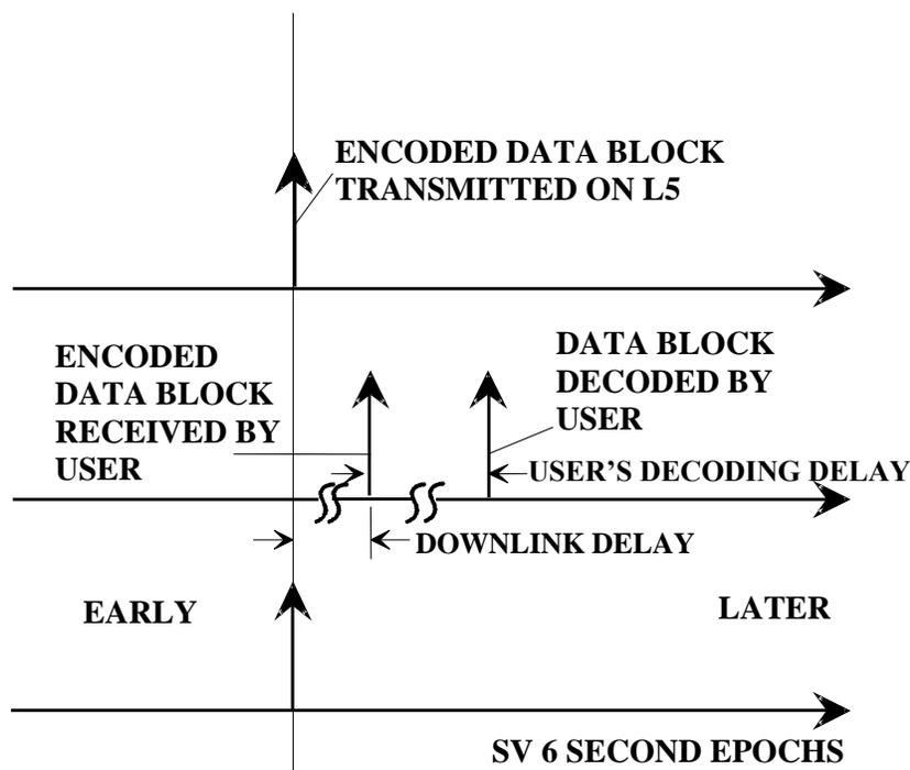
Figure 3-8. Convolution transmit/Decoding Timing Relationships
