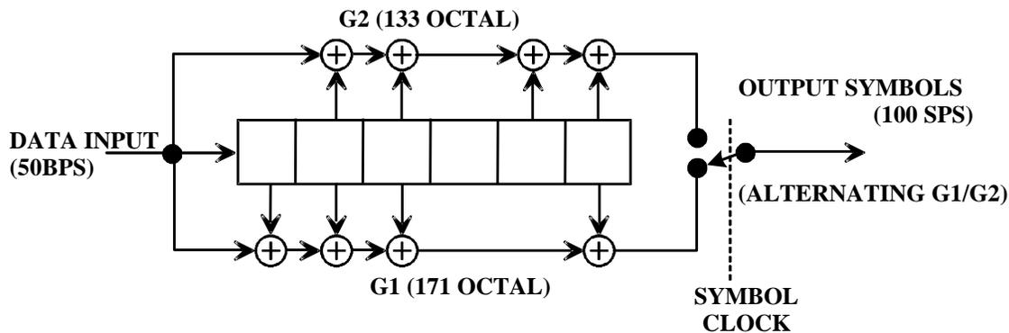
Figure 3-7. Convolution Encoder
