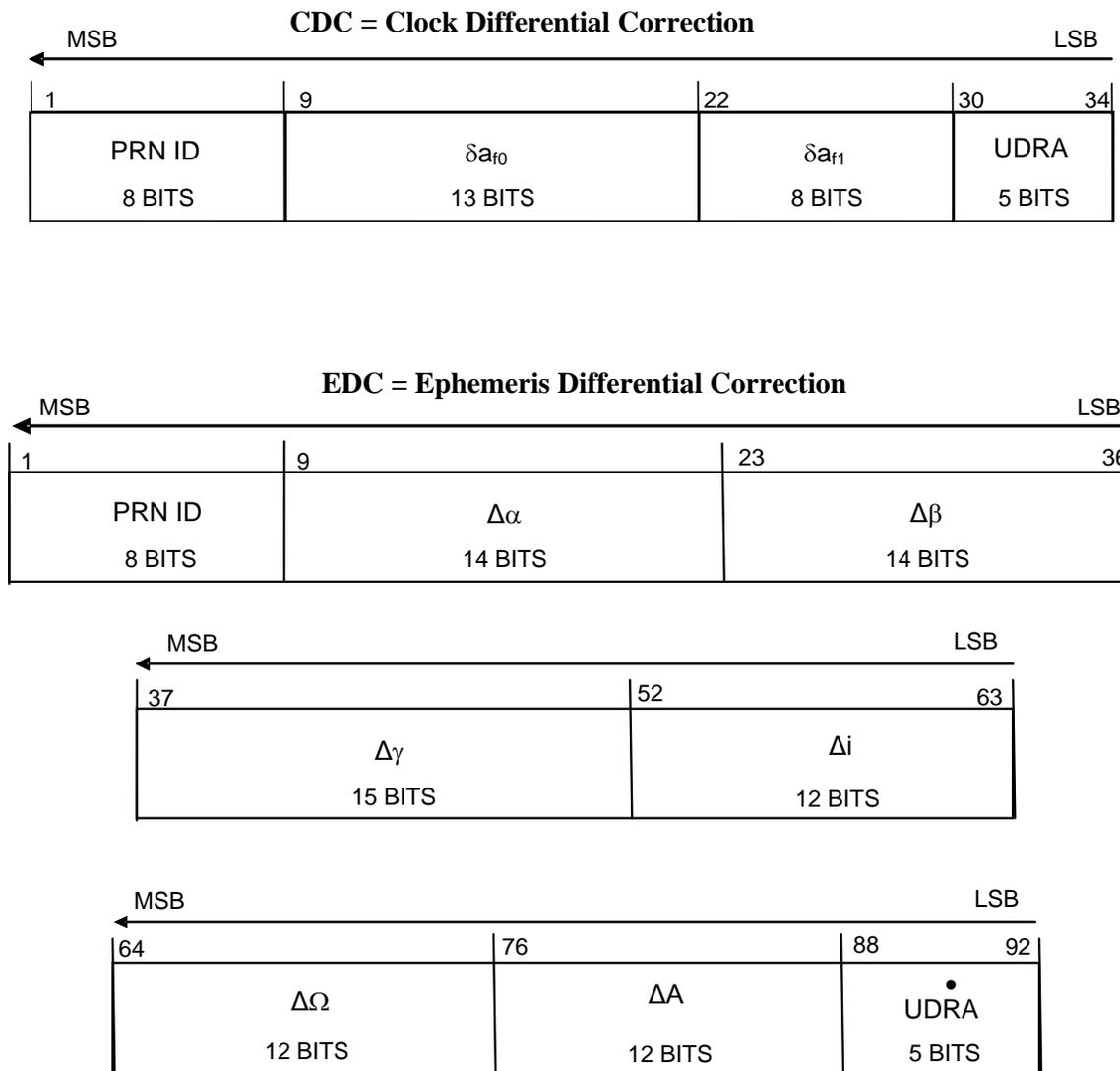
**Figure 20-17. Differential Correction Data Packet**
