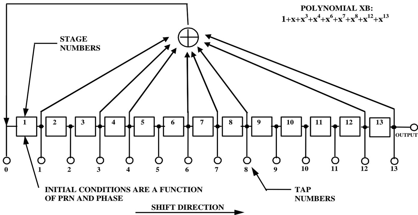
Figure 3-5. XB Shift Register Generator Configuration
