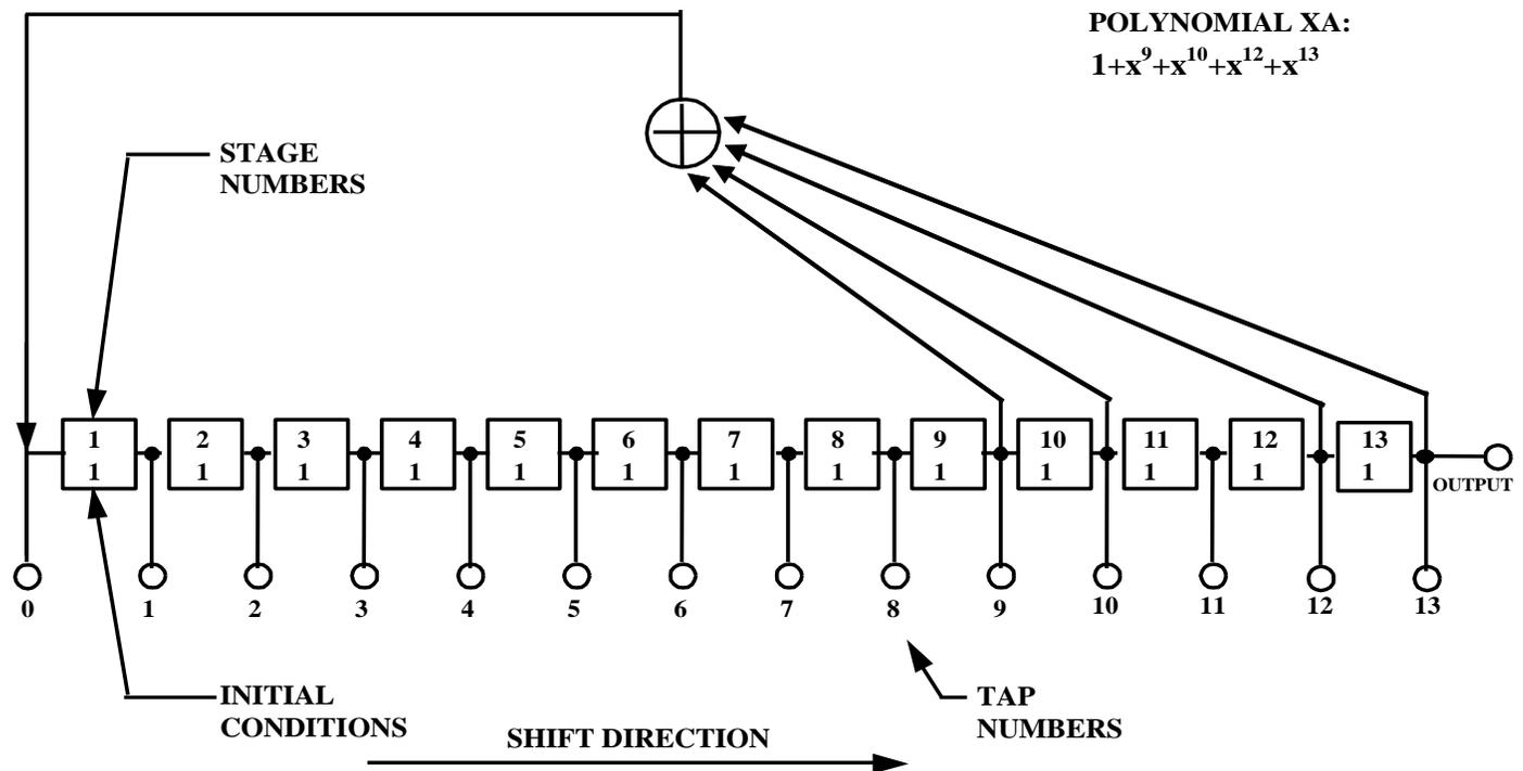
Figure 3-4. XA Shift Register Generator Configuration
