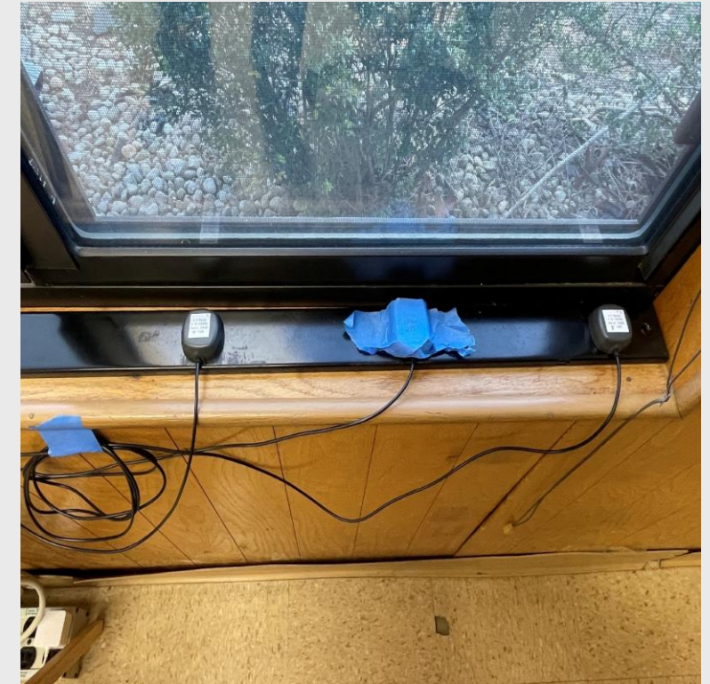
Two antennas (white sticker) for the Otosphere, one antenna (blue) for the u-Blox F9P
