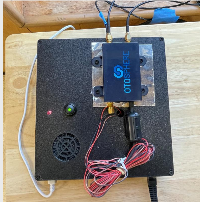
“Brain” consist of a Raspberry Pi, a u-Blox F9P, and an Infinidome Otosphere (gen-1) Jamming Mitigator
