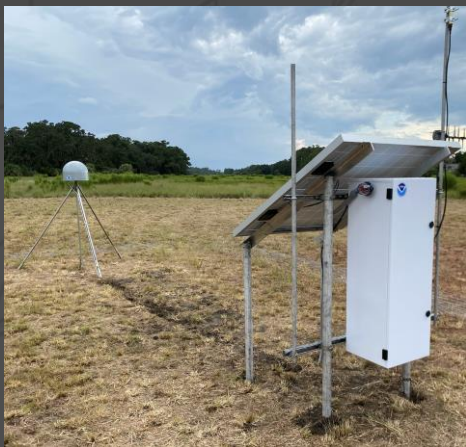
Complete Geodetic monument (antenna at top)
