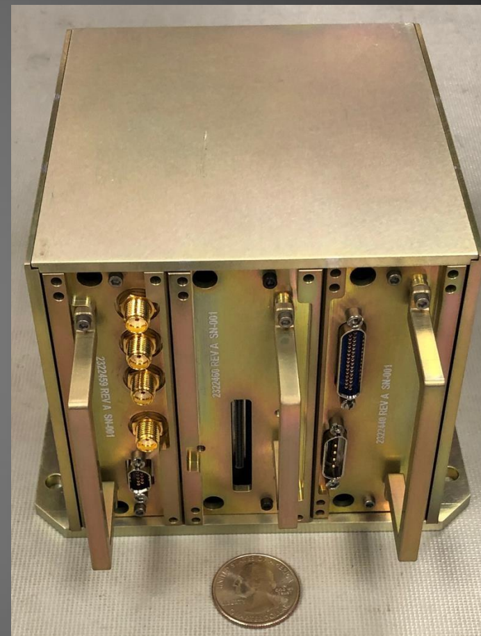
GPS Receiver Assembly
