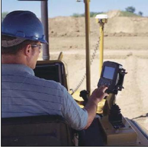
“According to Tom DiGiampaolo, operations manager, an operator on the company's Cat D6M was grading **two building pads per day following stakes**. But after fitting the machine with an automated GPS system, the operator cuts **six pads per day, minimum, with no stakes and no rework.**” – Construction Equipment, April 2004
