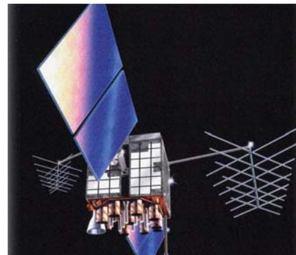
Block IIF satellites are the next generation of GPS space vehicles. Block IIF provides all the capabilities of the previous blocks with some additional benefits. Improvements include an extended design life of 12 years, faster processors with more memory, and a new civil signal on a third frequency (L5). The first Block IIF satellite is scheduled to launch in the near future.
