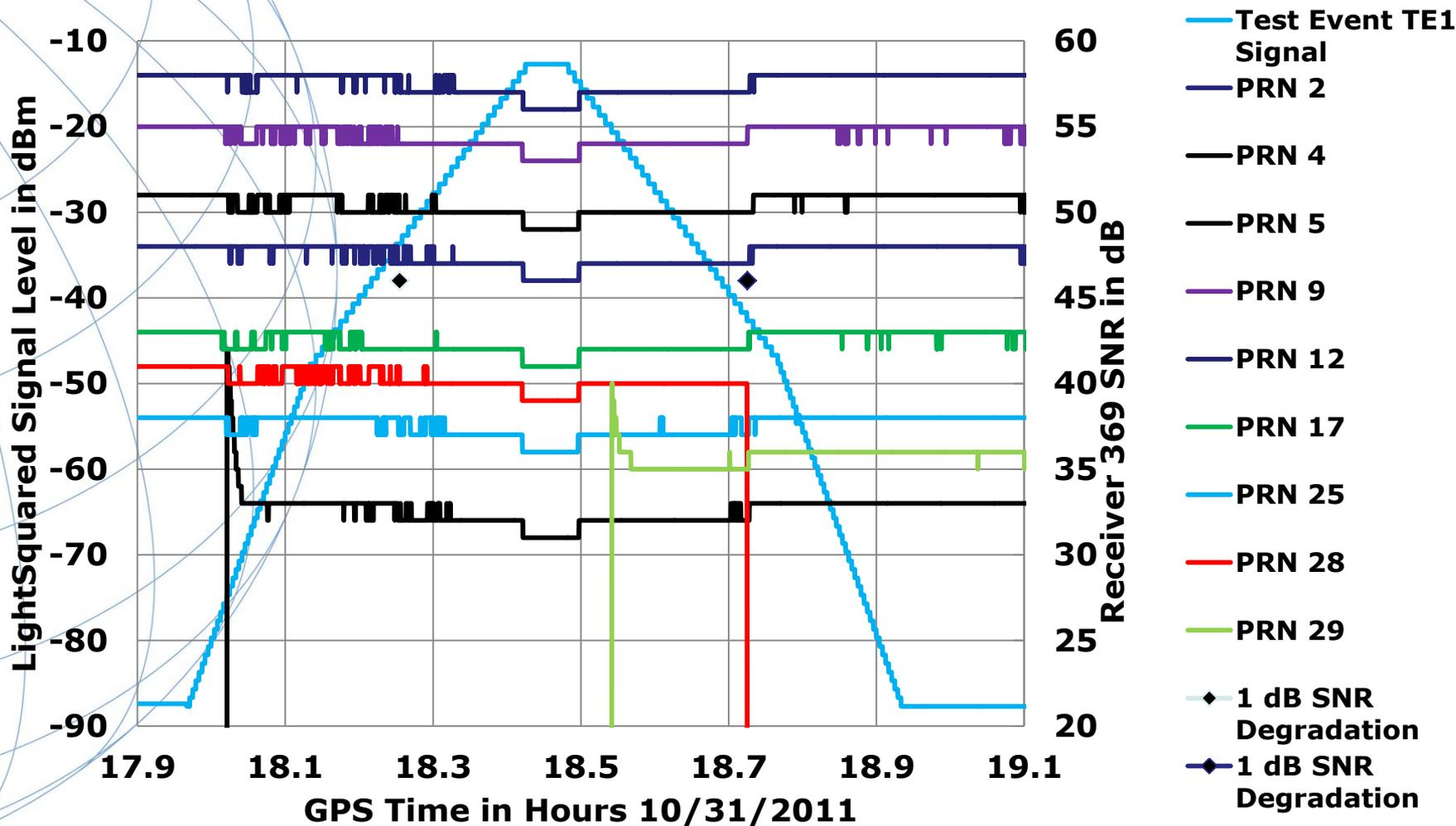
Receiver 369 / Ant. # 369 / Radial Position Error / Test Event TE1
