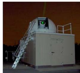
NASA SLR 2000 laser transmitter
