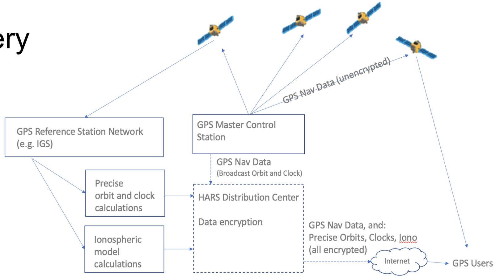
Data encryption and delivery block diagram for a High Accuracy and Resilience Service (HARS).
