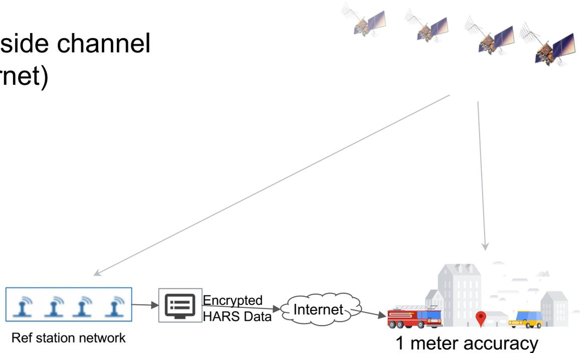
User accuracy with HARS: 1m, horizontal. 95% for patch antennas (e.g. cars), 50% for phones.
