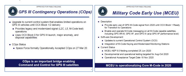
GPS III satellites are being controlled by the Contingency Operations (COps). This platform was accepted in March 2020. We needed to operationally accept this prior to entering GPS III SVs 01 and 02 into the operational constellation. This is an interim solution until delivery of OCX Blocks 1 and 2.
