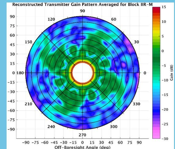
Block IIR-M reconstructed pattern from GPS ACE [11]
