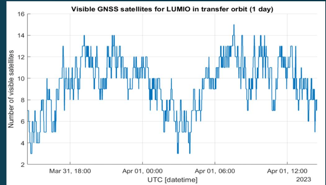
*Visible GNSS satellites for LUMIO over transfer from LLO to NRHO [11]*
