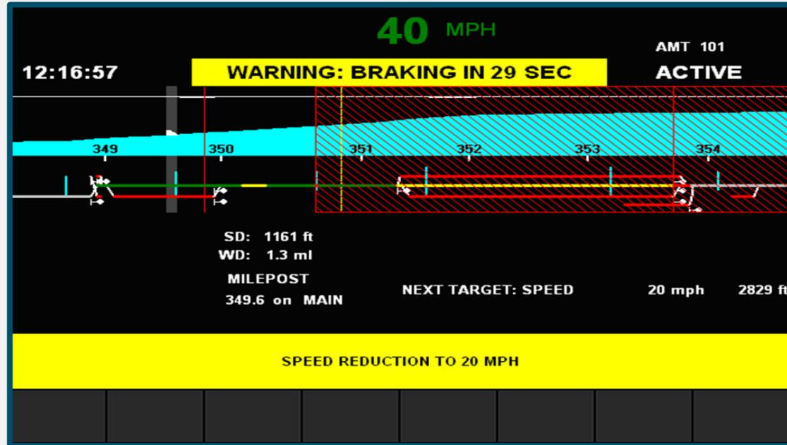
*If a train comes within Warning Distance of a speed restriction, and I-ETMS predicts train speed will exceed speed limit by 5mph or more when the train enters the restriction, a "Speed Reduction To XX mph" message will display along with the time remaining to enforcement braking.*
