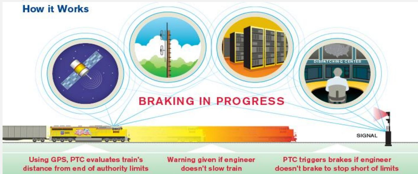
PTC MUST reliably and functionally prevent train-to-train collisions, overspeed derailments, incursions into established work zone limits, and movements of trains through switches in the wrong position.
