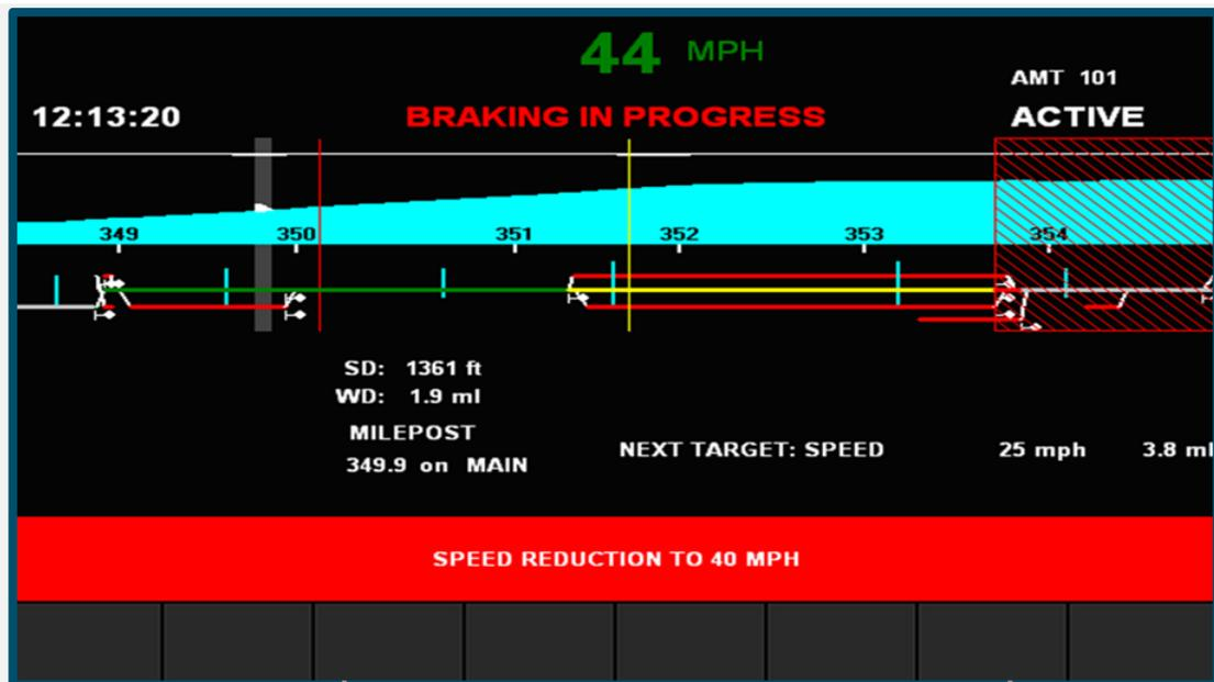
*If a train exceeds maximum speed allowed for the track by 3 mph, I-ETMS will display a warning to indicate the train is over speed and a “Maximum Speed Is xx MPH” message.*
