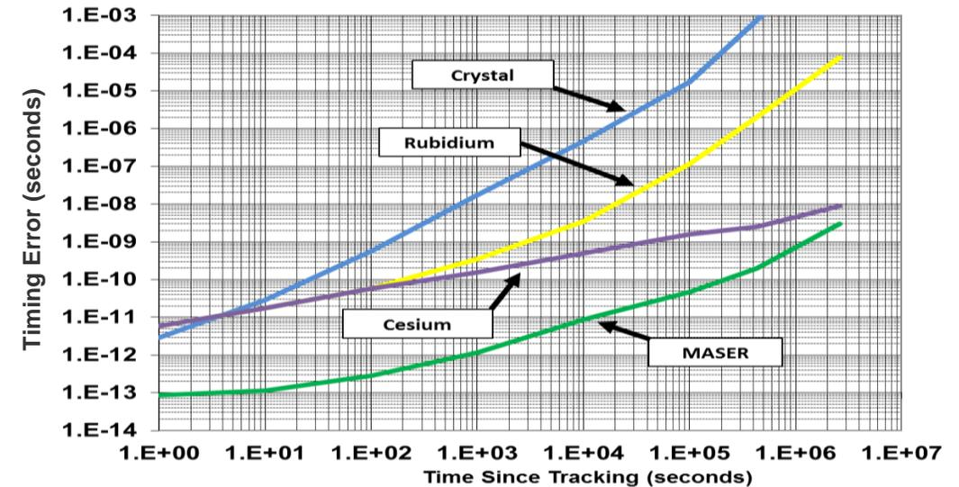
**Oscillator Type Determines How Long A System Can Operate Without GPS**
