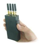
1 Watt-class jammers are small devices typically used for jamming personal location devices in commercial industries. They have a limited range and are typically battery operated.
