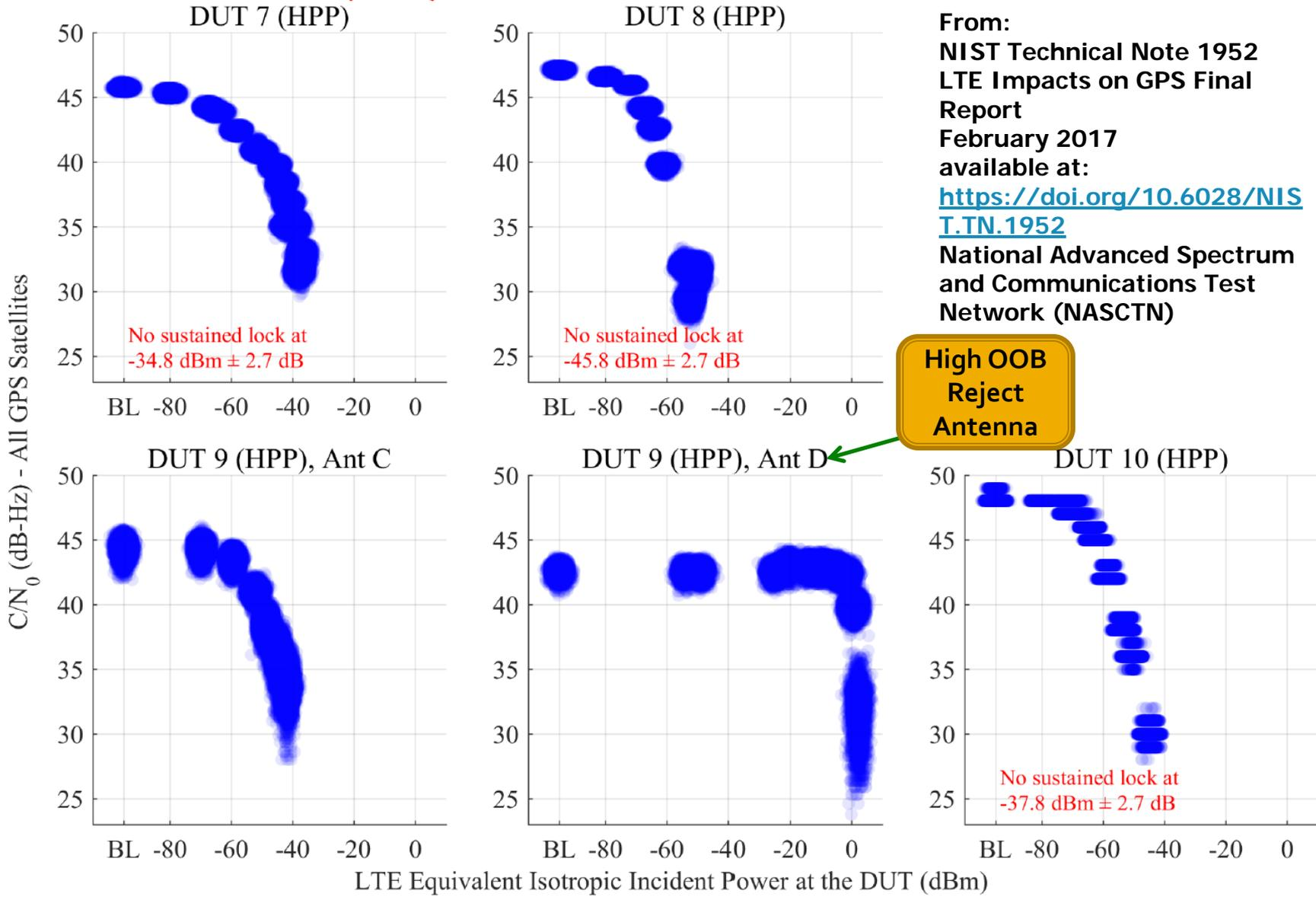
Figure 6.24: Scatterplots of reported  $C/N_0$  from HPP receivers, swept with LTE power level. The GPS scenario is nominal, and the type of incident LTE is DL.
