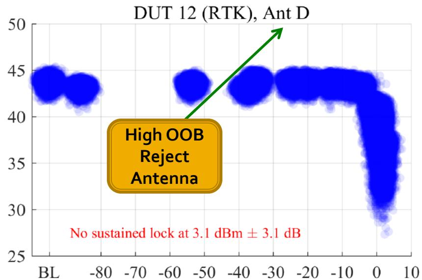
LTE Equivalent Isotropic Incident Power at the DUT (dBm)
