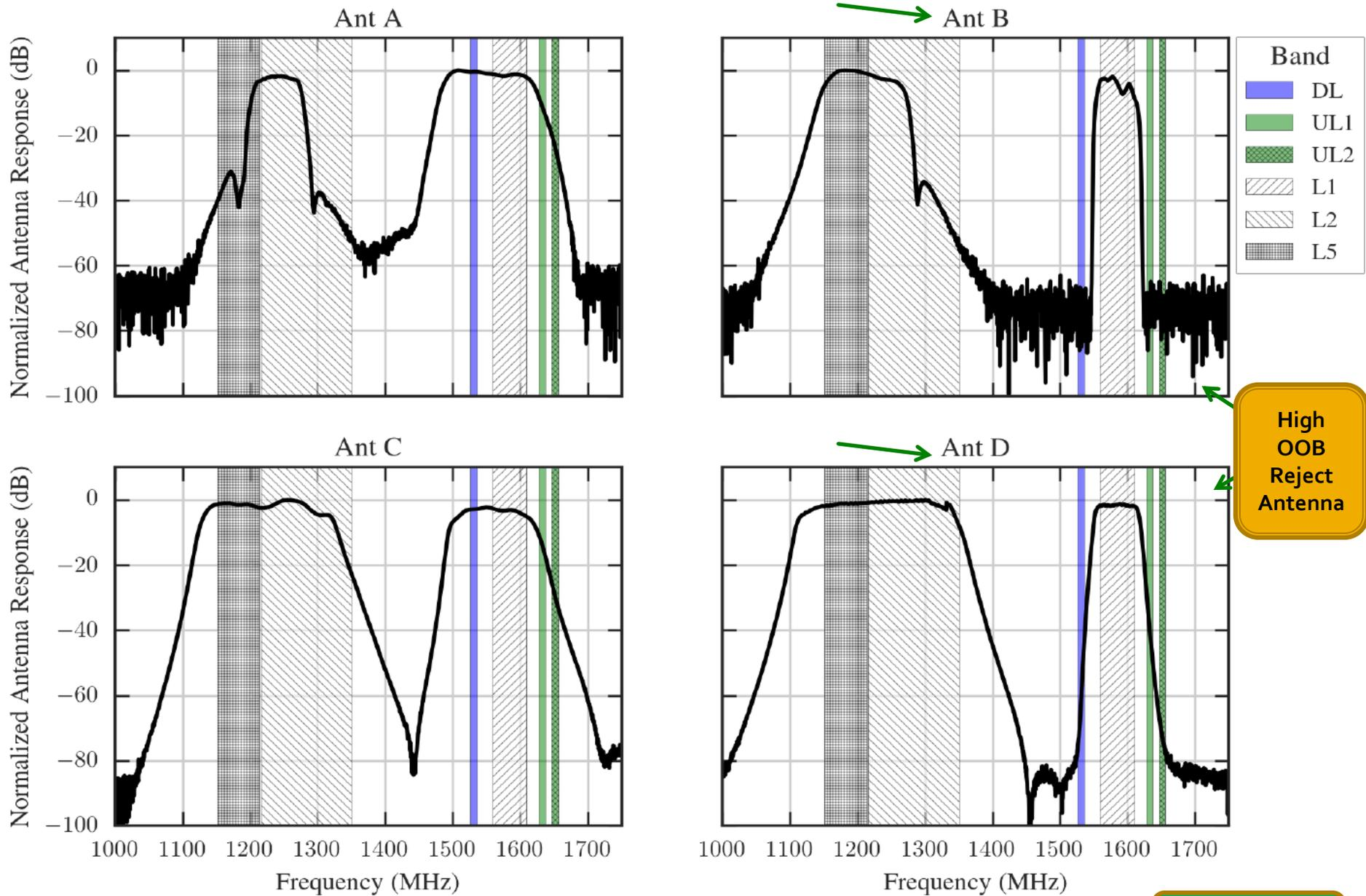
Figure 6.2: Normalized  $S_{21}$  S-parameter responses of external DUT antennas.
