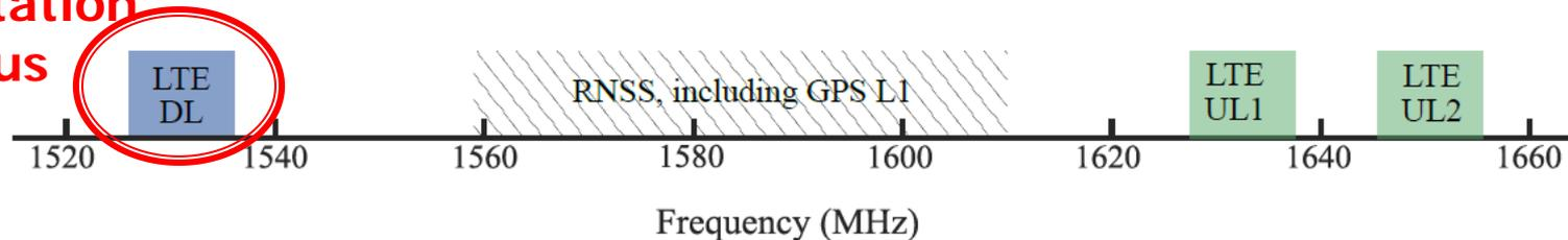
Figure 1.1: Spectrum allocations showing RNSS, which includes the GPS L1 band, and the various adjacent bands proposed for LTE use.
