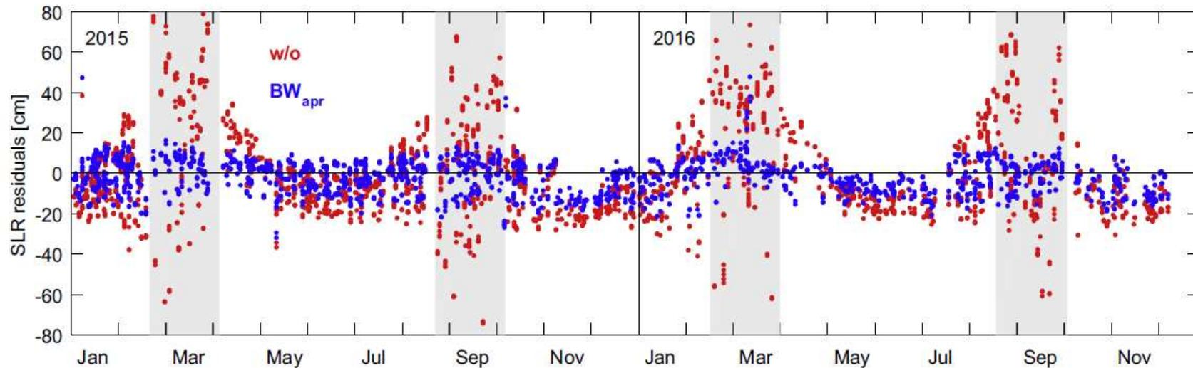
Fig. 8. Satellite laser ranging residuals (gray: without a priori model; blue/red: with a priori box-wing model in YS/ON mode). The gray shaded areas indicate time periods with ON mode. (For interpretation of the references to color in this figure legend, the reader is referred to the web version of this article.)
