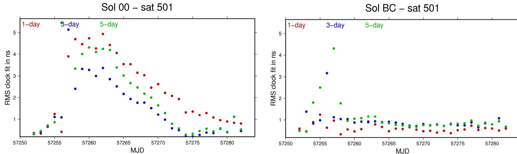
**QZS-1 moving under ON-Mode from MJD=57256 onwards, Sun in orbital plane for MJD=57275, 1-, 3-, and 5-day solutions.**
