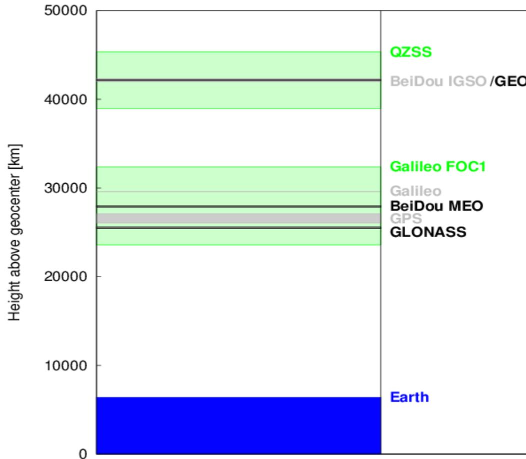
Close to **100 GNSS & RNSS** satellites have different characteristics (semi-major axes  $a$ , eccentricities  $e$ , inclinations  $i$ ) and different signals, tracking modes.
