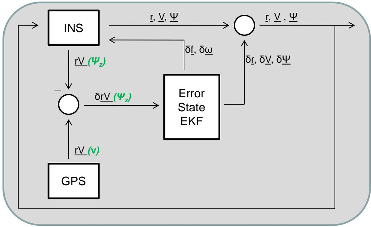
$$Y = \begin{bmatrix} \underline{r} \\ \underline{V} \\ \psi_{yaw} \end{bmatrix}_{GPS} - \begin{bmatrix} \hat{\underline{r}} \\ \hat{\underline{V}} \\ \hat{\psi}_{yaw} \end{bmatrix}$$
