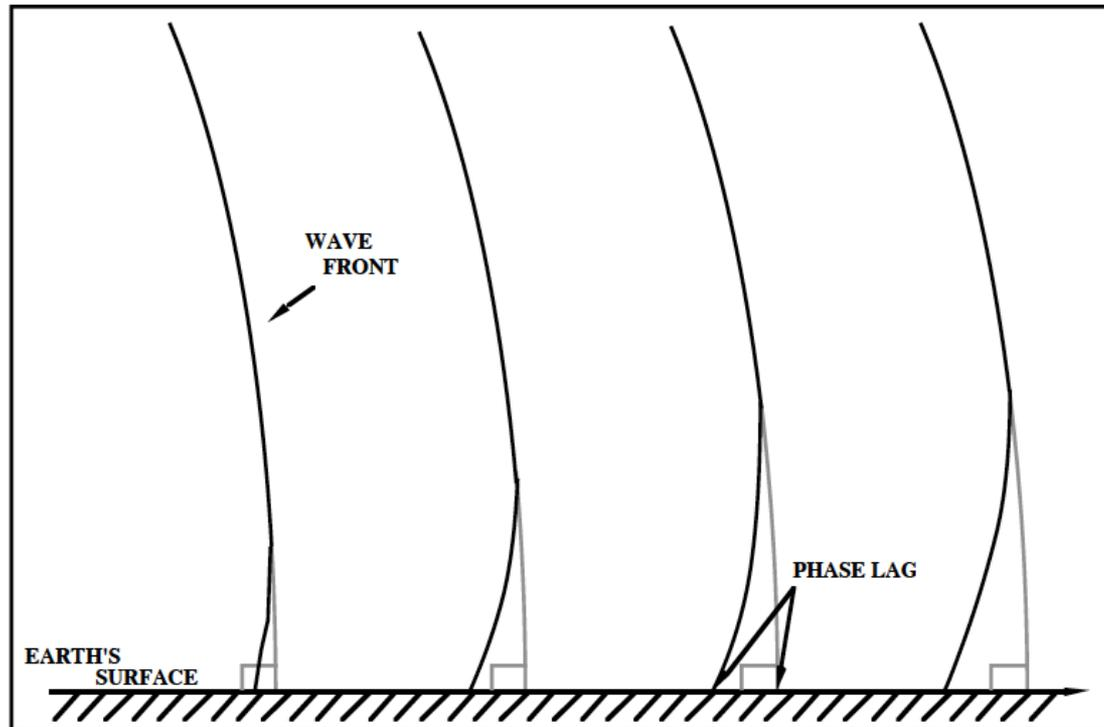
**Figure 2: Loran phase lag**
