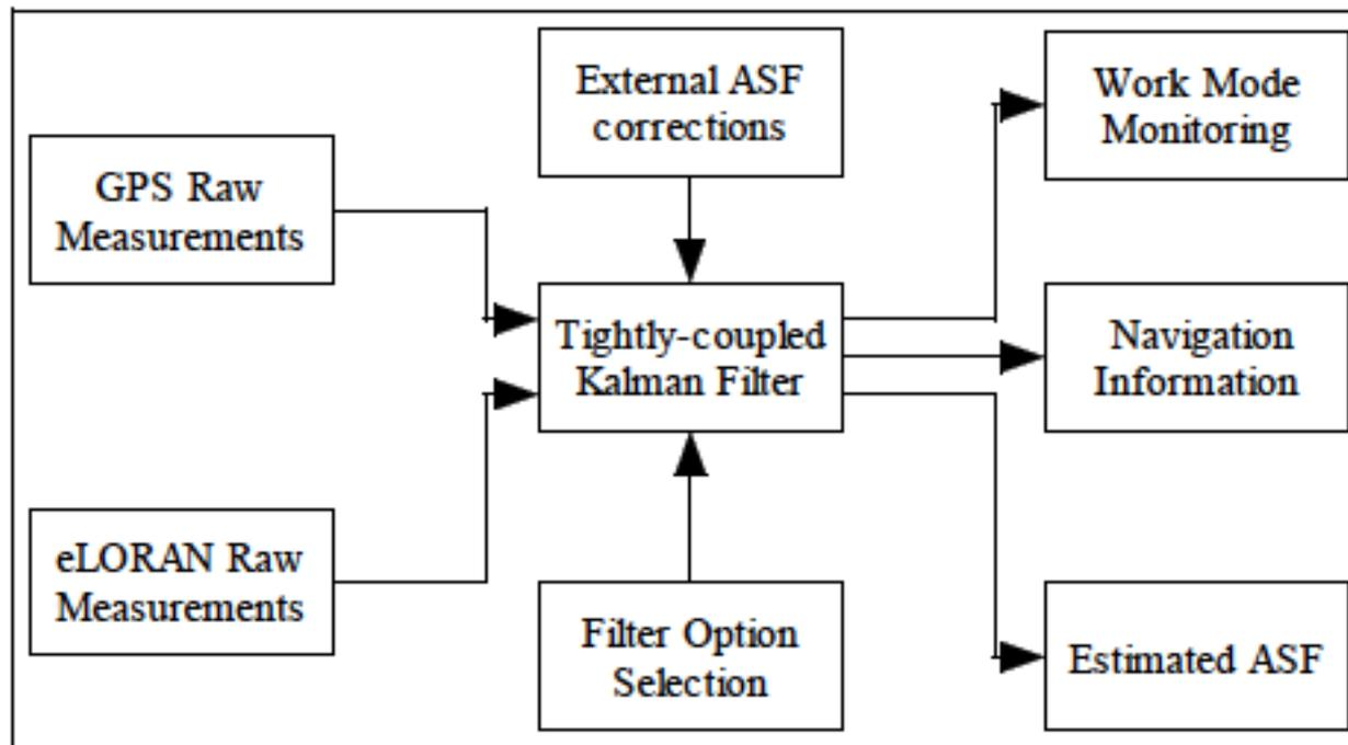
**Figure 11: Structure of an integrated GPS/eLORAN system**
