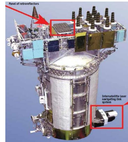
Figure 1. Panel of retroreflectors and Intersatellite laser navigating link system at the SC «GLONASS-M».
