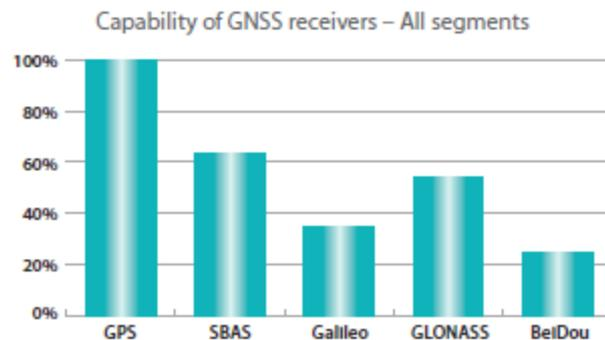
The **"Capability of GNSS devices"** chart shows the percentage of available receivers capable of tracking the SBAS, GPS, Galileo, GLONASS and BeiDou constellations. GPS is naturally present in all devices, followed by GLONASS. Galileo and BeiDou are progressively adopted by the leading manufacturers. In some cases, the full capability of GNSS receivers (chipsets/modules) is not necessarily used in the products/devices (e.g. SBAS capability in LBS segment).
