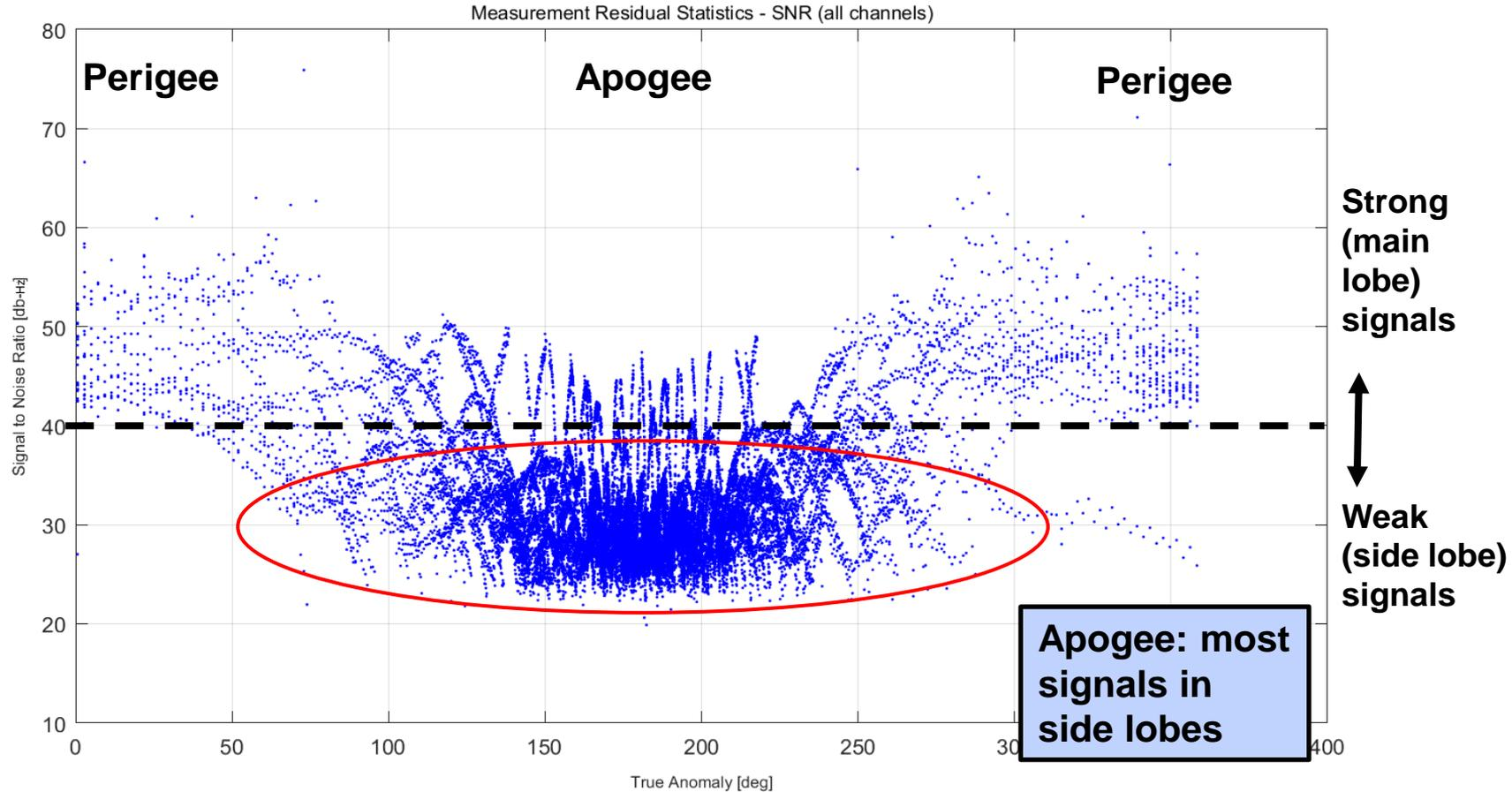
**Signal strength (C/N0) vs. position in orbit**
