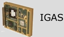
Digital Beam Former High-AJ GPS
