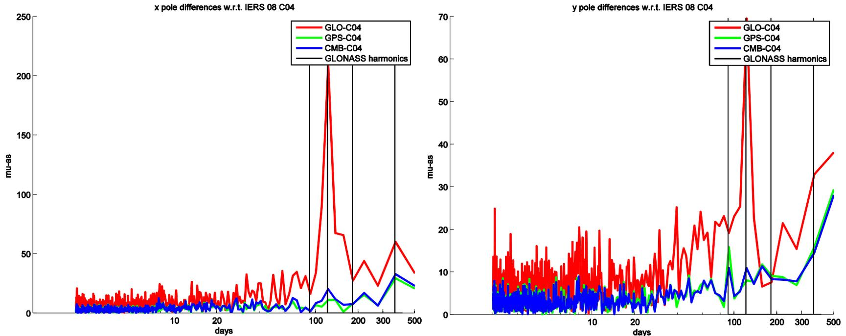
**Polar motion components x & y compared to IERS 08 C04.**
