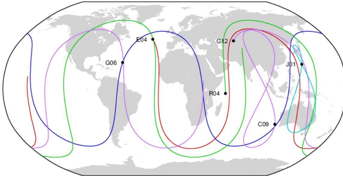
Daily Groundtracks of **GPS**, **GLONASS**, **Galileo**, **BeiDou**, **QZSS** (geosynchronous, GPS augmentation).
