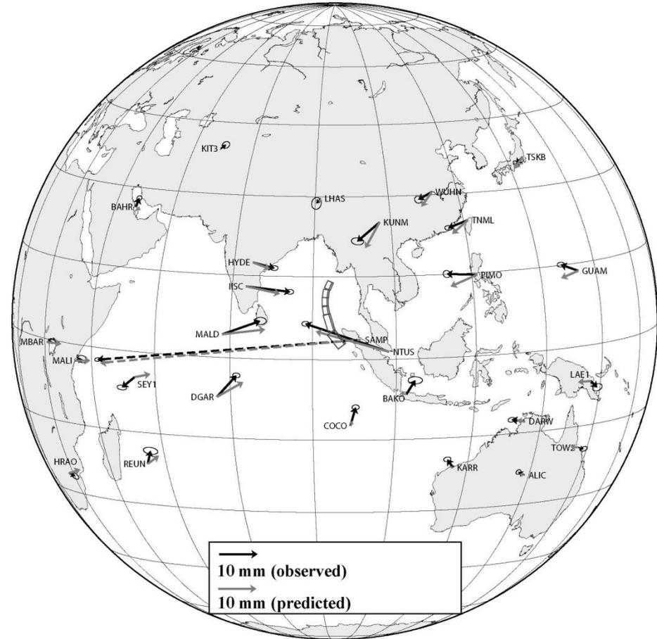
GPS station displacements on 26 December, 2004 observed by the International GNSS Service Network (IGS/GGOS). The largest arrow (SAMP) has been scaled down by a factor of two for clarity.
