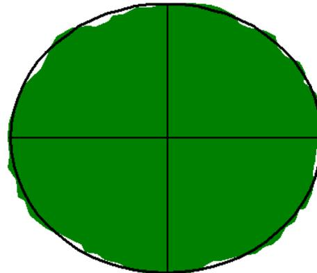
The geoid is used as a surrogate for mean sea level, the vertical datum for traditional 'elevations'
