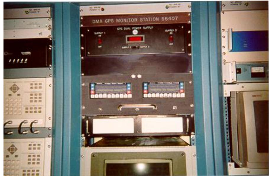
The NGA GPS Tracking Station at USNO uses a frequency standard tied to UTC(USNO)
