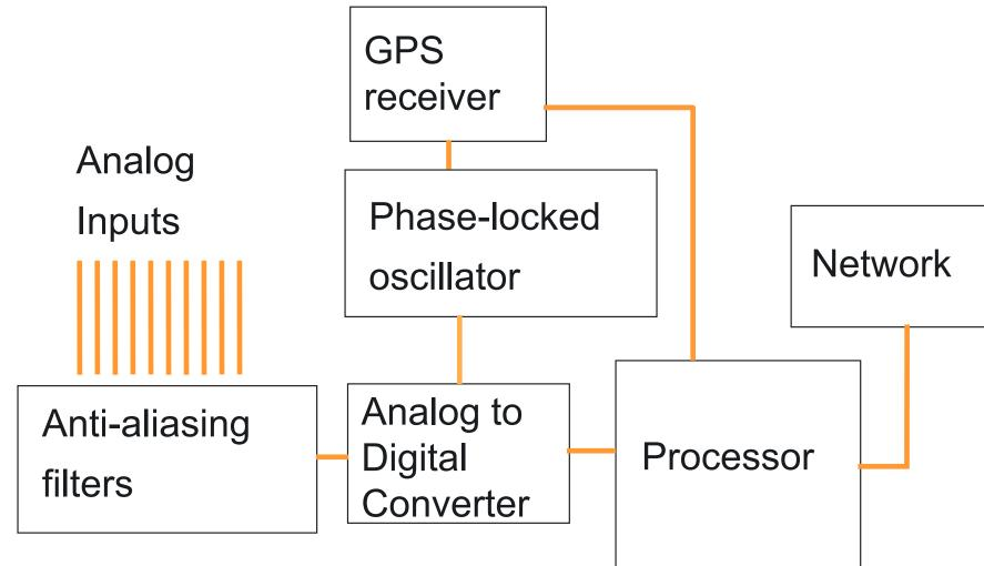
Except for synchronization, and some post processing, the hardware is the same as that of a digital fault recorder or a digital relay.
