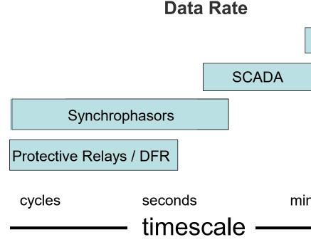
Time synchronized data can be gathered at reporting rates much faster than traditional supervisory control and data acquisition (SCADA) systems
