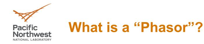
• A phasor *represents* magnitude and phase angle of a sinusoidal wave
