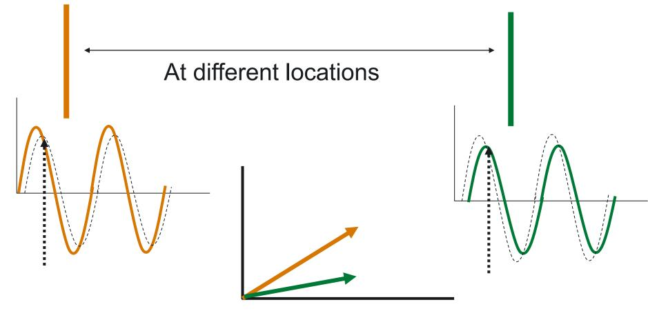
By synchronizing the sampling processes for different signals, which may be hundreds of miles apart, it is possible to put their phasors on the same phasor diagram.
