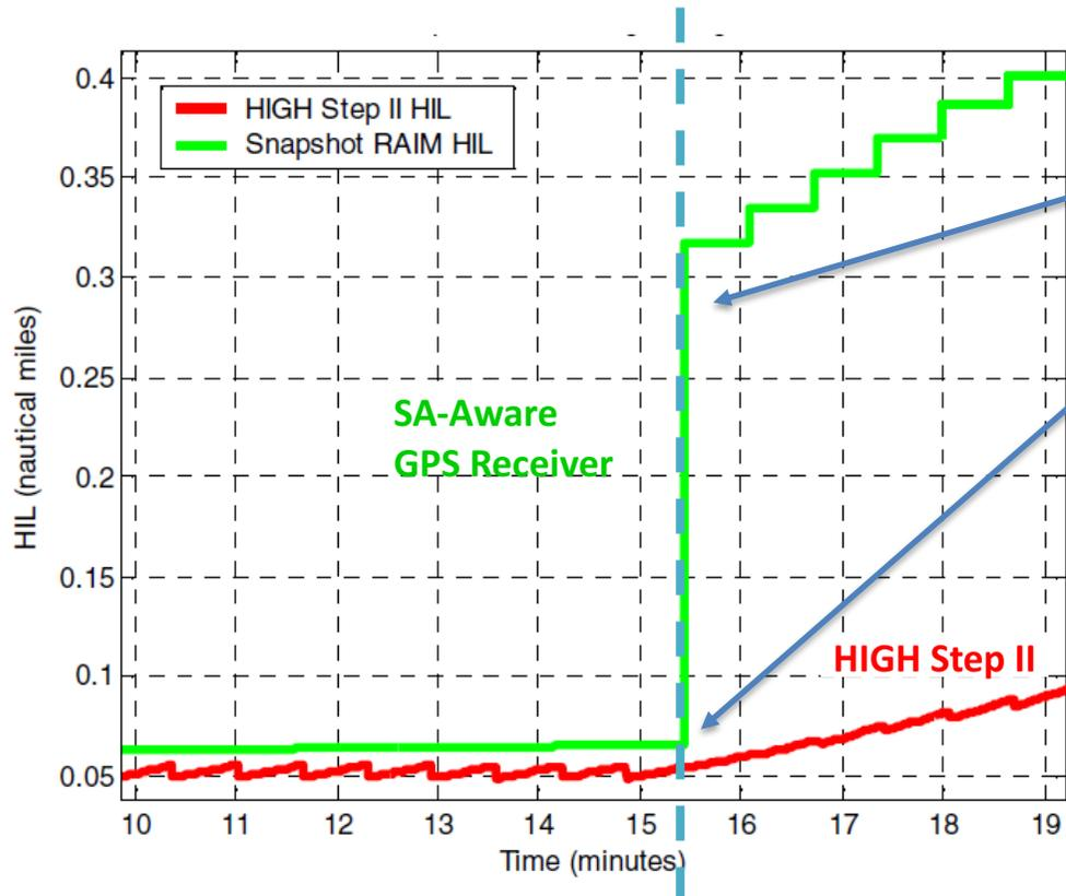
Upon entry into this RAIM hole just after T = 15 min, the GPS Receiver HIL instantly responds to the degraded satellite geometry
