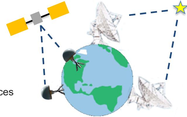
A current geodetic research frontier is co-locating observing instruments for multiple techniques, and measuring the baselines between them with goal of supporting  $\sim 1\text{mm}$  absolute accuracy,  $\sim 0.1\text{mm/year}$  drift
