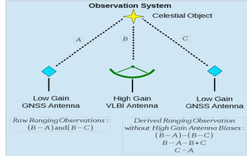
*The goal is measurements of the baselines at reference frame co-location (fundamental) sites directly through the instruments*
