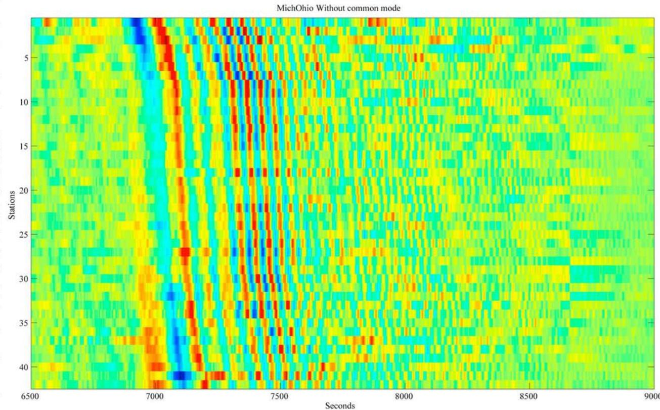
We can estimate wave properties such as apparent velocity and azimuth by array processing (beam steering, fk filtering).
