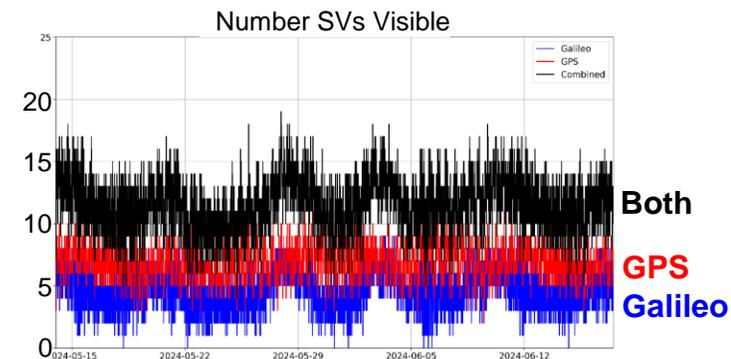
**Predicted Gateway GPS/Galileo visibility (20 dB-Hz; courtesy ESA)**
