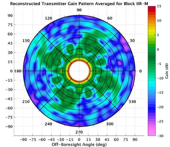
**Block IIR-M reconstructed pattern from GPS ACE**
