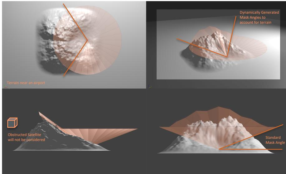
During an approach, the terrain is different on every point along the trajectory and is dynamically derived if required.
