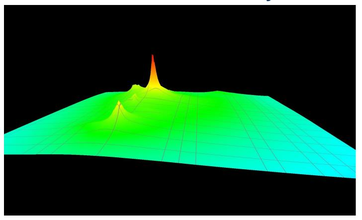
Probability density "heat map" example generated by real case of ADS-B track gaps due to RFI (Method developed by Valeriu Vitan, EUROCONTROL)
