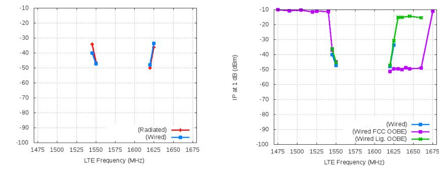
Radiated and wired 1 dB ITM's in good agreement consistent with expectations since both tests used device filter/LNA
