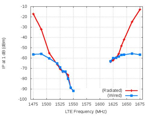
Antenna not characterized but Filtering evident in comparison of radiated and wired 1 dB ITM's
