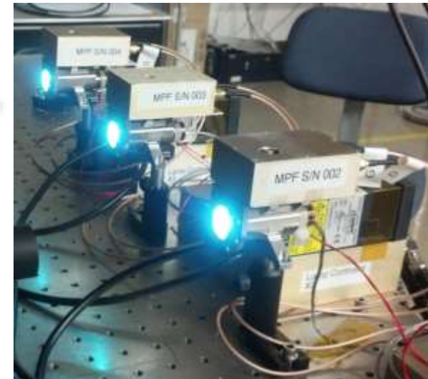
Mercury UV Lamp Testing
