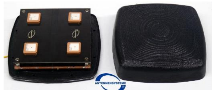
GPS/Galileo E1 (miniaturized, analog frontend integrated)
