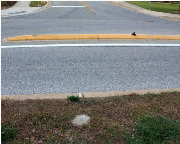
UMBC SURVEY CONTROL 1 st order survey markers Set in place by Frederick Ward surveyors in 2007
