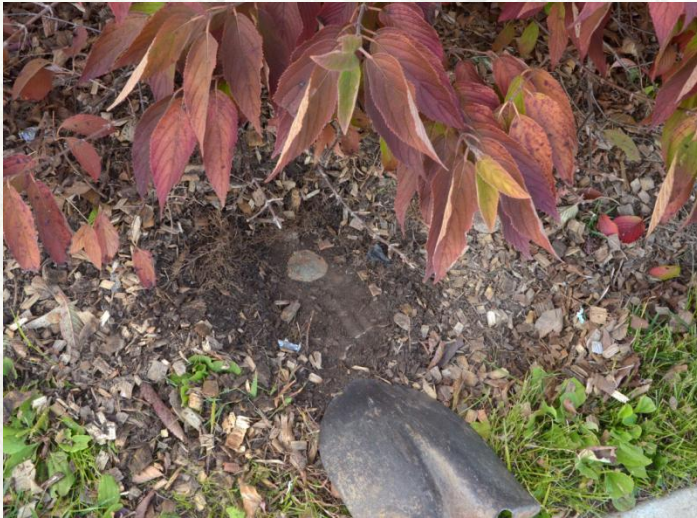
UMBC SURVEY CONTROL 1 st order survey markers Set in place by Frederick Ward surveyors in 2007
