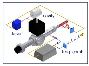
schematic of thermal beam optical clock
