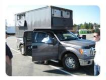
A custom enclosure was built tall on a large pickup truck to afford the 14 synchronized cameras a clear view of the roads and road rights of way. The truck uses GNSS receivers as well as ground targets to georegister the millions of images it collects and stores in on-board solid-state-drive servers. From the collected and registered images, high precision photo-interp positions can be extracted for all visible roadside features.
