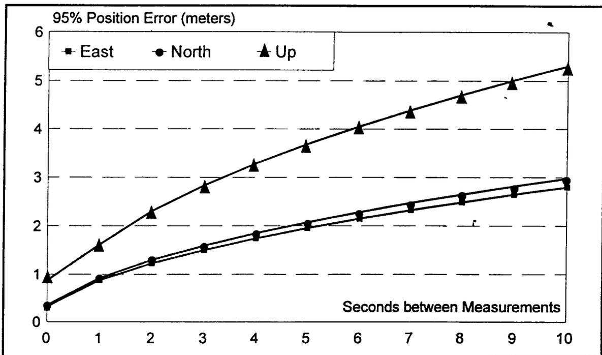
Figure 5-9. Relative Accuracy as a Function of Time Between Position Estimates
