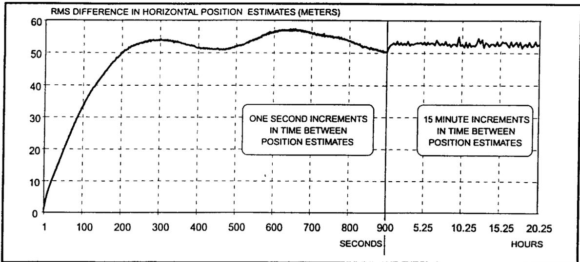
Figure 5-8. Repeatable Accuracy as a Function of Time between Position Estimates
