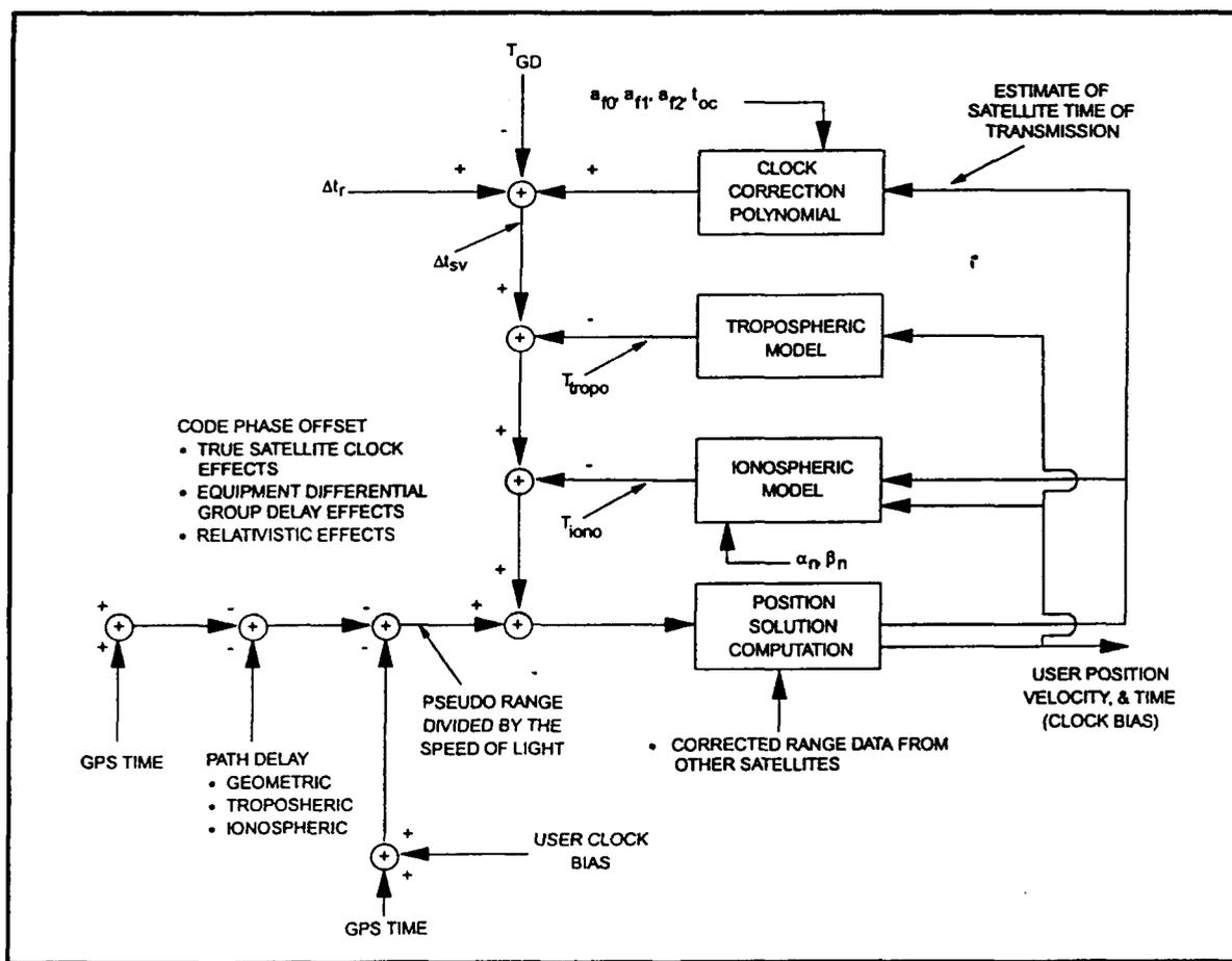
Figure 2-11. Application of Correction Parameters
