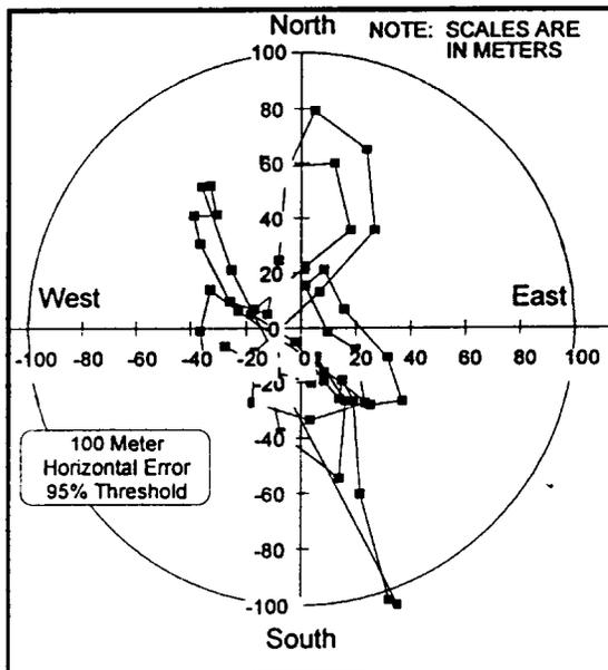
Figure 5-1. Horizontal Errors over 1 Hour
