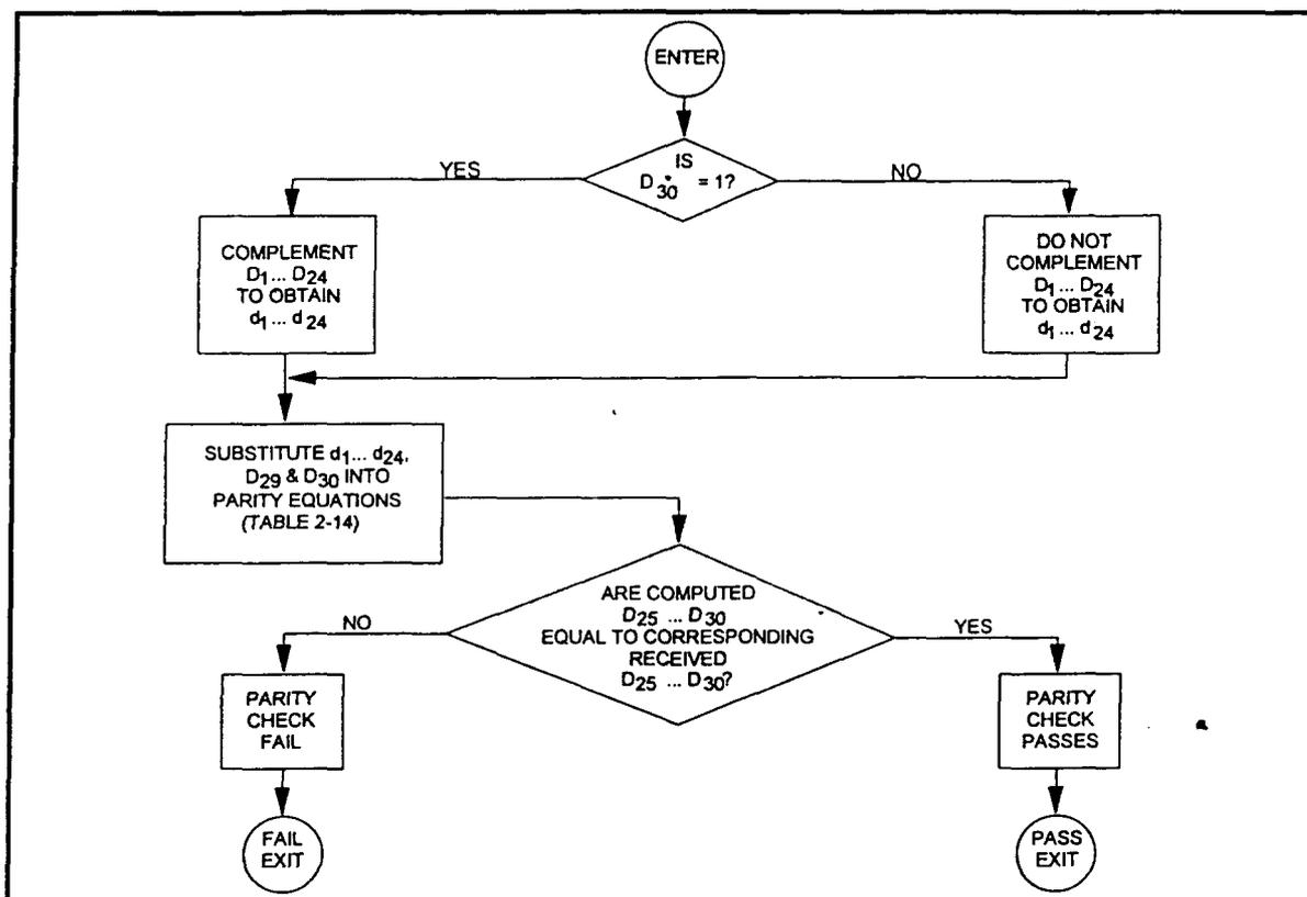
Figure 2-10. Example Flow Chart for User Implementation of Parity Algorithm
