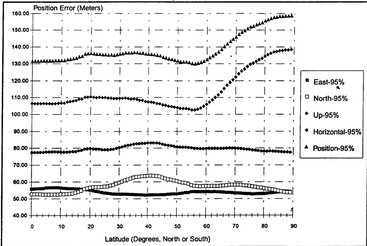
Figure 5-5. GPS Accuracy as a Function of Latitude
