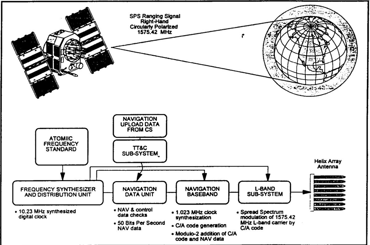
Figure 1-1. SPS Ranging Signal Generation and Transmission
