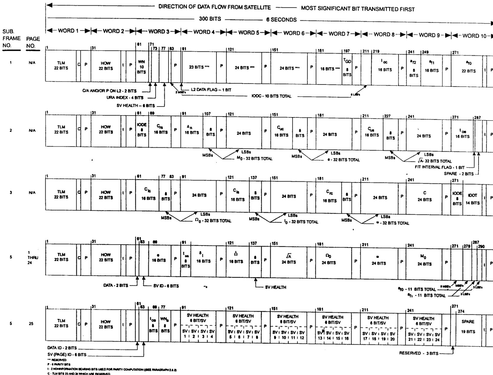
Figure 2-8. Data Format (Sheet 1 of 2)
