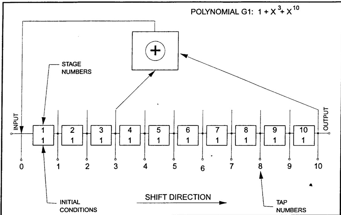
Figure 2-2. G1 Shift Register Generator Configuration
