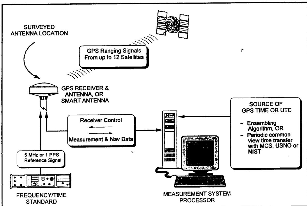
Figure 3-1. Example of Type 3 Measurement System Configuration
