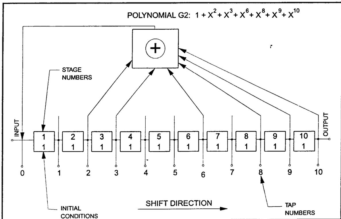
Figure 2-3. G2 Shift Register Generator Configuration
