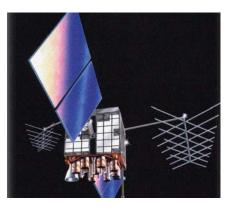
satellite processors enabling problem fixes and upgrades in flight. Eight Block IIR satellites are being modernized to radiate the new civil signal (L2C) on the L2 channel. The first modernized Block IIR (designated as the IIR-M) with L2C was launched on 26 September 2005.
