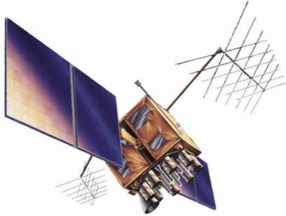
GPS network measures plate tectonic motions to an accuracy of better than 1 mm/yr
