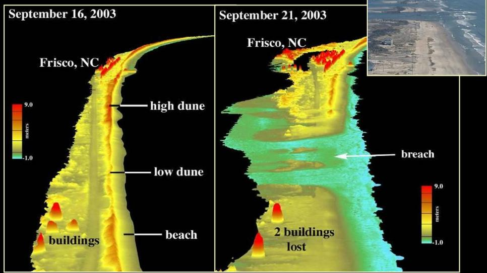
**GPS Dependent Airborne Lidar Mapping Enables Understanding of Coastal Change Hazards**
