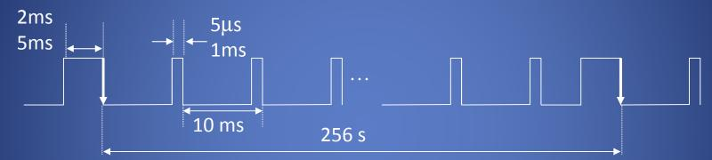
The relative phase difference of the synchronization Signal shall not exceed 2.5 μs (3 μs is mentioned for TD-SCDMA) External sync Source (e.g. GPS)
