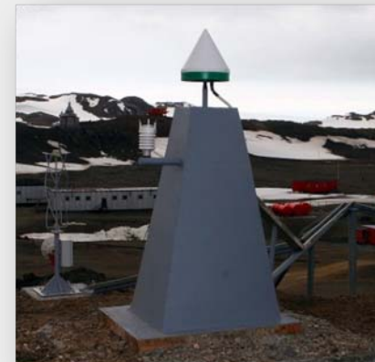
GLONASS/GPS antenna + Vaisala weather station
