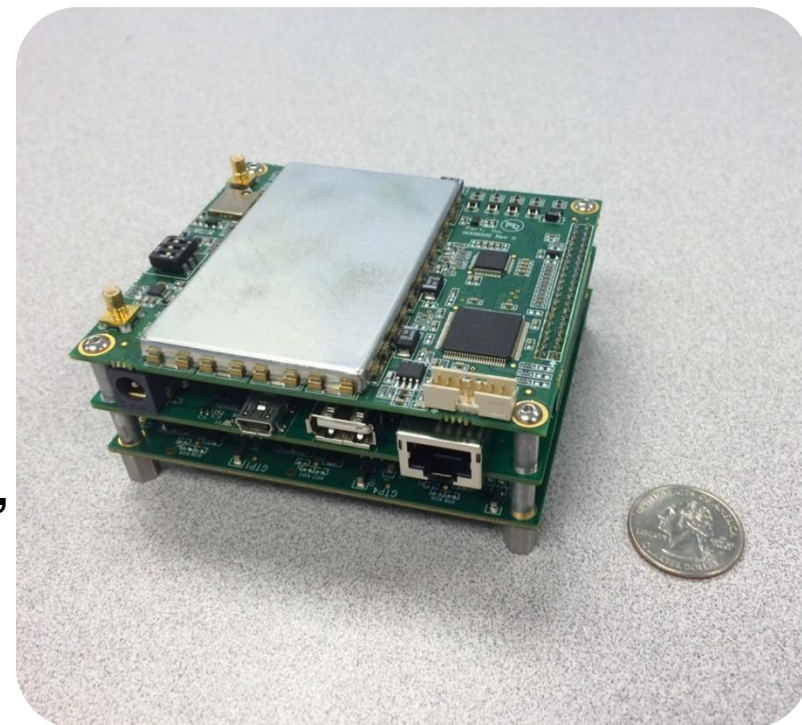
GAMMA GPS Receiver: RFE, on-board DSP and SBC interface unit
