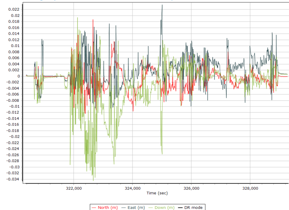
Smoothed Best Estimate Trajectory – inertially aided kinematic ambiguity resolution forward/reverse separation
