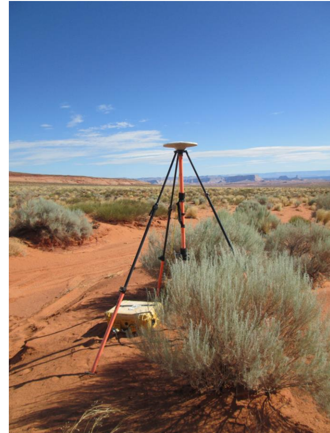
GNSS reference station (base station) outside LeChee Arizona
